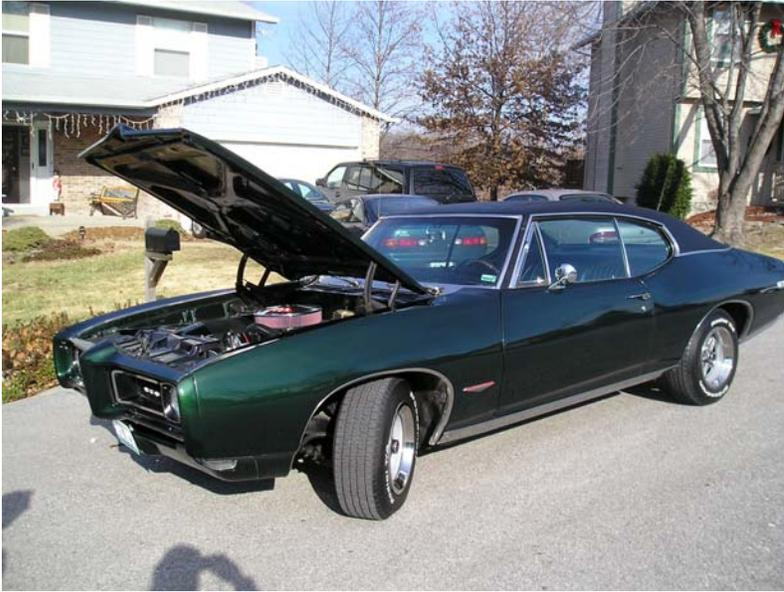
This past winter and spring some modifications were made under the hood and to the rear of the car. My mechanic, Randy Bardle, found a 428 engine he thought I needed. Between Randy and Bob Stiegemeier, the 428 was reworked with forged pistons, roller rockers, different heads and a Ram Air exhaust manifold. A MSD electric system was installed along with a Stiegemeier racing carb
